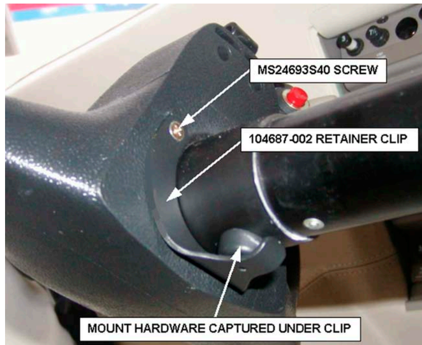
Control Wheel Installation Figure 1
