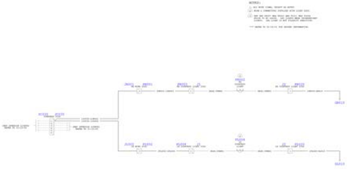
Figure 02 : Sheet 01 : UNDER WING COURTESY LIGHTS
