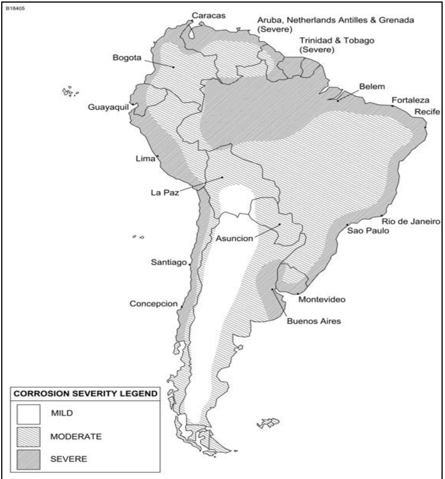
Figure 3 : Sheet 1 : South America Corrosion Severity Map
