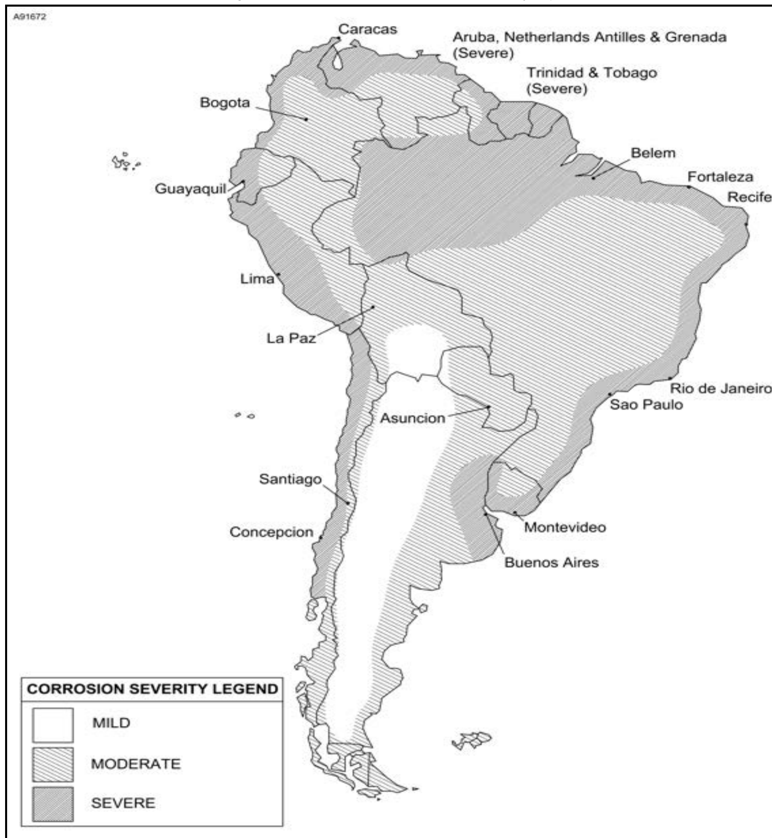
Figure 2 : Sheet 1 : South America Corrosion Severity Map
