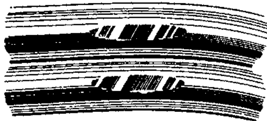
INDIVIDUAL OUTER WIRES WORN LESS THAN 40 PERCENT (WORN AREAS INDIVIDUALLY DISTINGUISHABLE)
