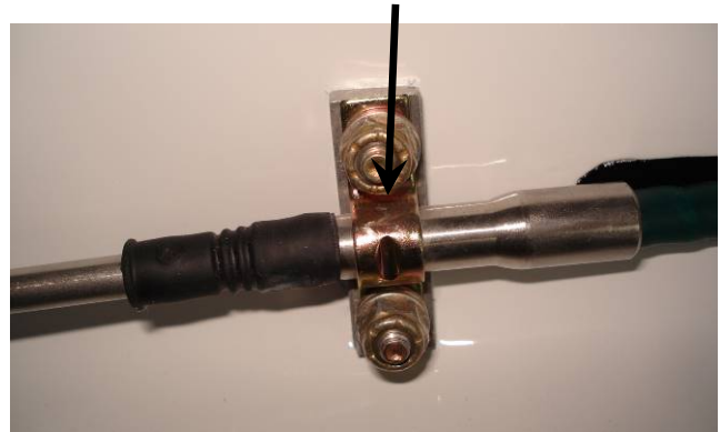
Figure 58 – Clamp Comparison & Installation (Rudder Cable)
