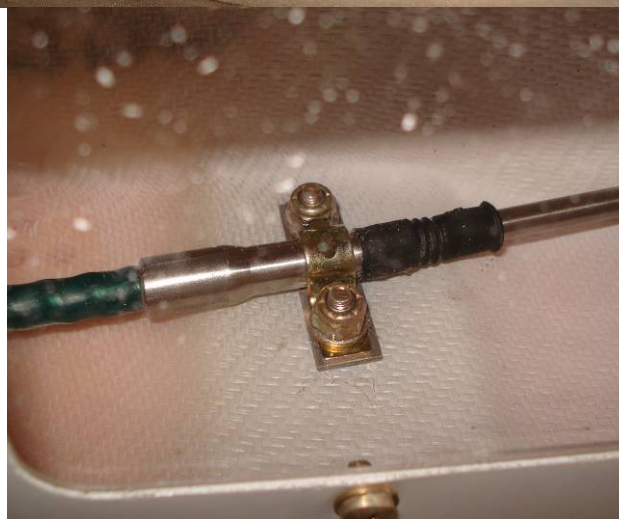
Figure 59 – Clamp Installations (Elevator & Aileron)
