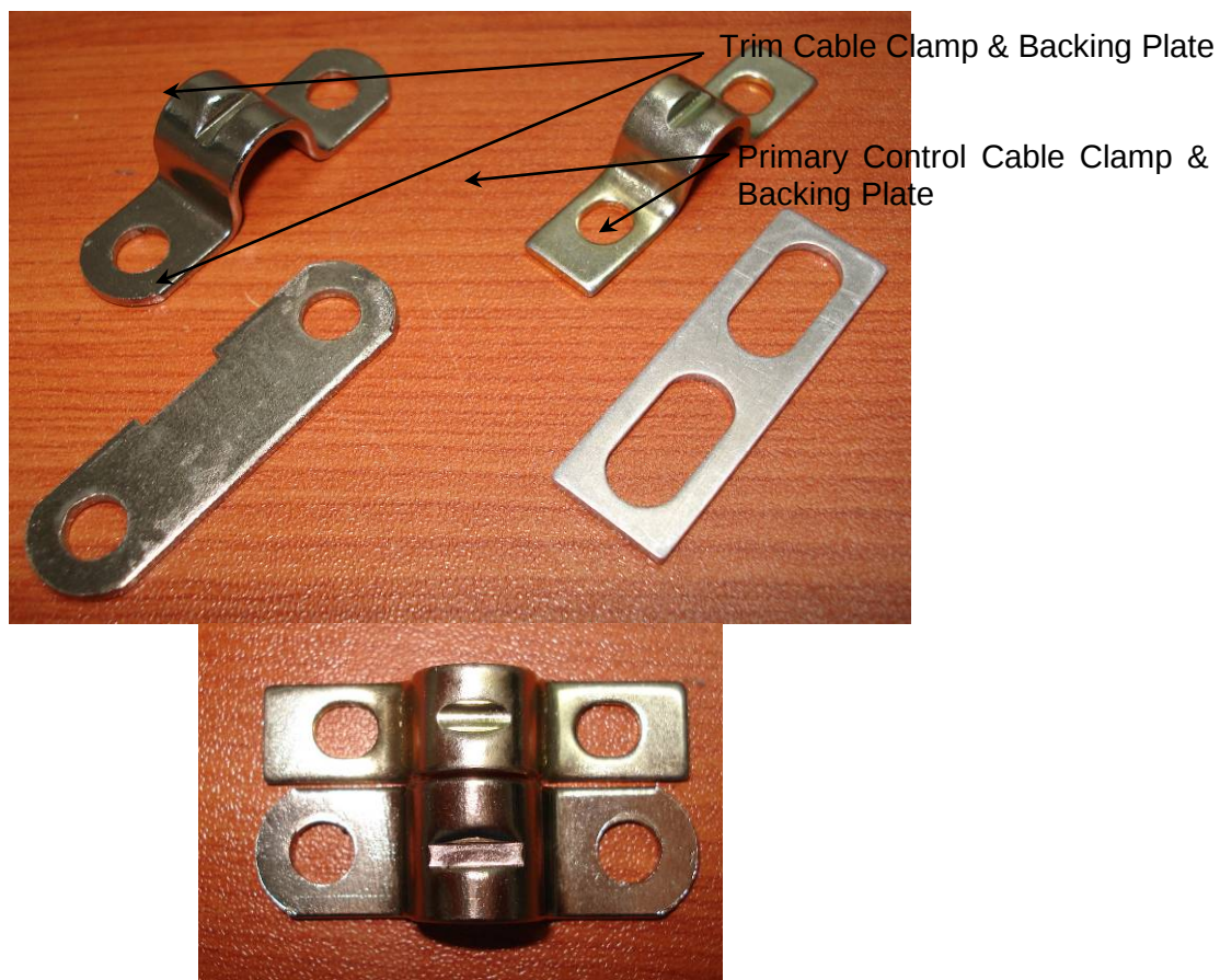
Figure 57 – Clamp Comparison (Primary Cable Clamp Upper on Right Picture)
