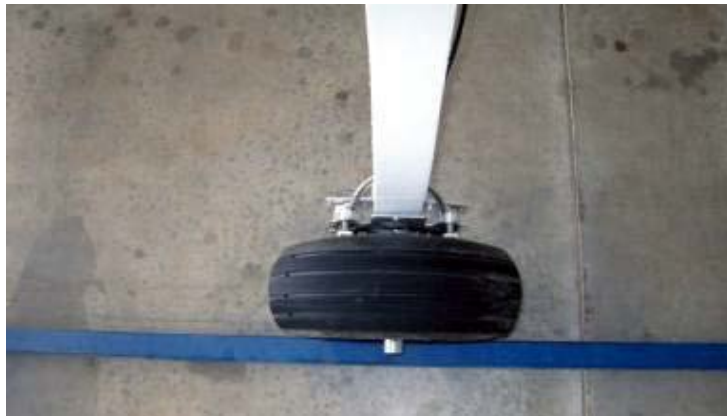
Figure 18 – Alignment Straight Edge In Position
