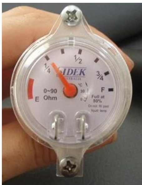
Figure 23 – 20L Indication on Sender & Decal to Match
