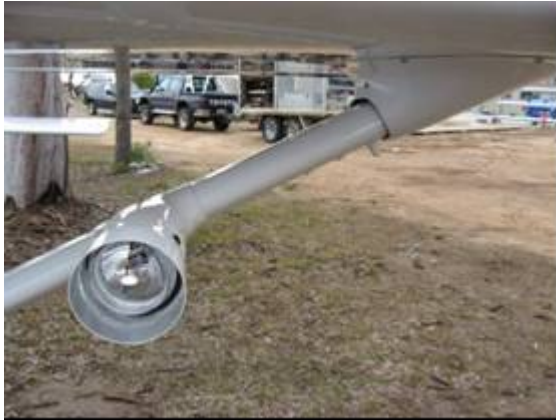
Figure 39 – Light Installed (Left) & Slotted Hole In Housing
