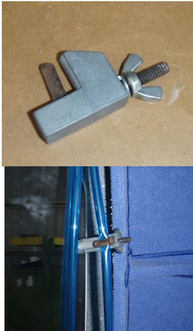
Figure 25 – Fuel Line Clamps
