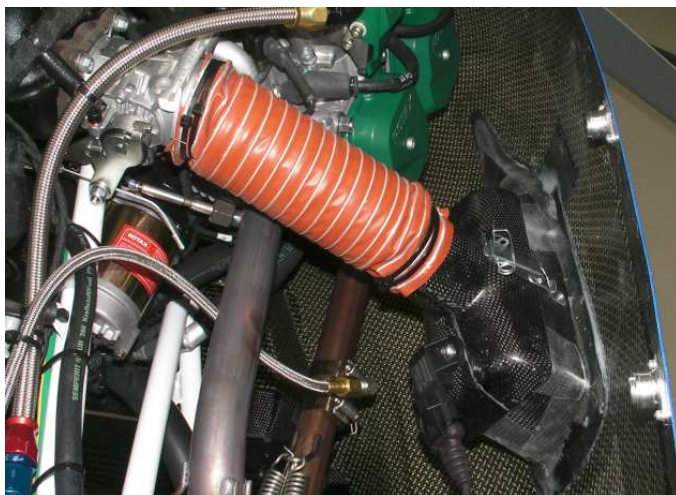
Fig. 10-20 Air filter installation on the lower cowling
