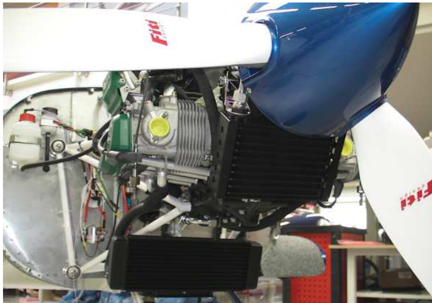
Fig. 10-18 Attachment of the radiator on the engine
