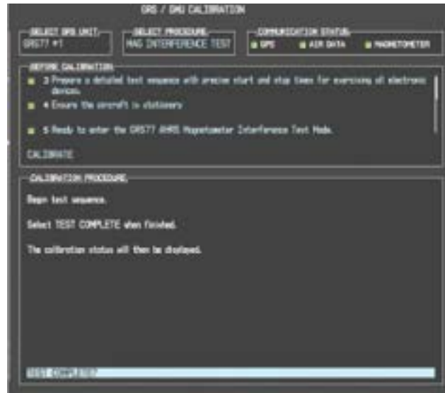
Magnetometer Interference Test Figure 37
