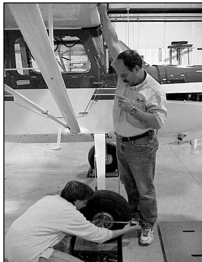
Figure 3-4, Measuring Datum to Main Wheel
