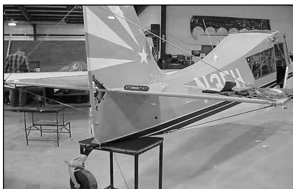
Figure 6-6, Attaching and Leveling Stabilizer
